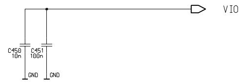
Decoupling capacitors for 1st flash
